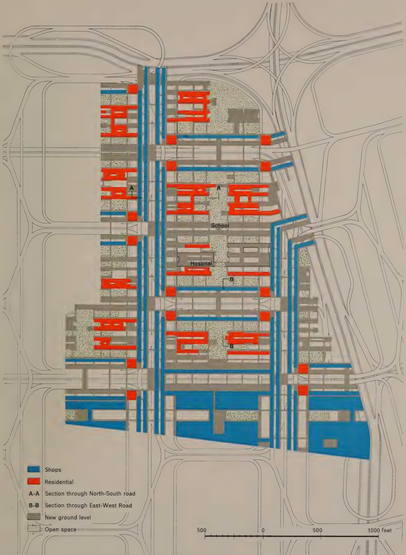
182 The design for complete redevelopment—plan showing the broad disposition of uses at deck level. Sections A-A and B-B refer to Figures 183 and 184. Areas on the new ground level which are not indicated for shops or residential use are for office, commercial and industrial purposes.
